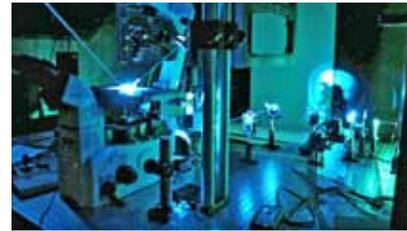
*Professor Wang has developed a new molecular imaging method using the laser system above, for single-particle tracking in biological systems. Her group aims at a better understanding of biological mechanisms at the level of single molecules by the investigation of protein-nonspecific DNA interactions at the base-pair level.*
