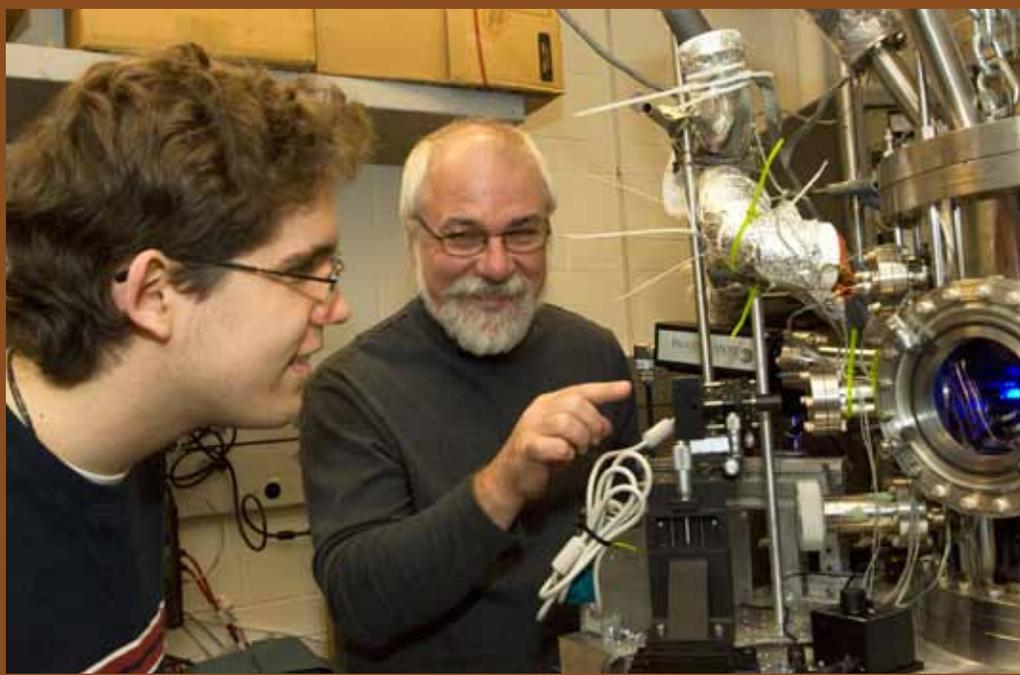
Professor Ken Kelton works with undergraduate physics major Austin Hope on structural studies of supercooled high temperature liquids using a novel electrostatic levitation technique.
